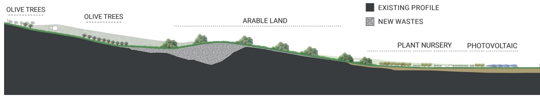
Figure 16.3.14 Cross section of the landfill. The wastes are used as a plastic material to shape the land. Graphics: Studio Arcoplan.
